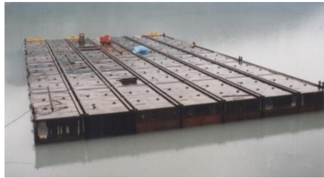
(a) Single unit pontoon (b) Hull assembled by 28 FBs
